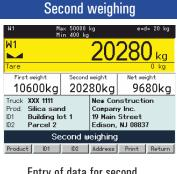
Entry of data for second weighing, display of first weight and net weight
