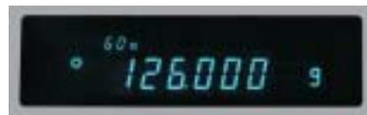
**Overall Capacity Indication** is a unique and helpful feature. By indicating how much of the balance's capacity has been filled, the risk of overloading the balance is minimized.
