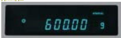
**Animal Weighing Mode** allows you to quickly and accurately determine the weight of any live or unstable subject. Optional animal weighing pan (GX-12) is available.
