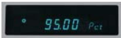
**Percentage Function** facilitates an effective and quick comparison of a sample or commodity against a known reference mass. Simply place an object on the pan to register its weight as 100%. Place another object on the pan to compare its weight in percentage mode.
