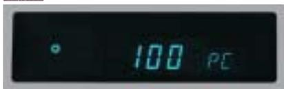
**Automatic Counting Accuracy Improvement (ACAI)** is a novel and useful approach to ensuring the utmost in performance when counting even the smallest of items. ACAI automatically updates and refines the average piece weight used to determine the total quantity.
