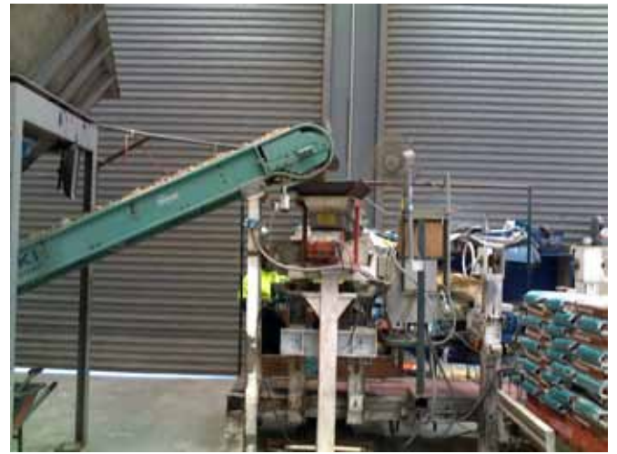
TWIN-HEAD (DENDY) VIBRATORY FED GROSS WEIGH BAGGING SCALES
