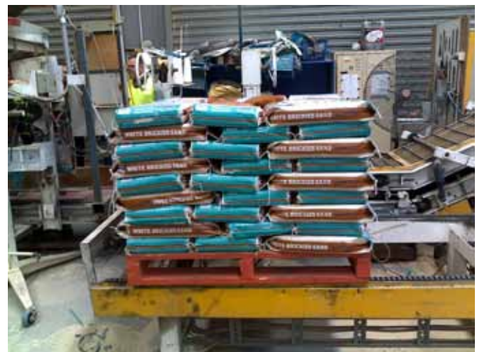
FILLED PALLET ACCUMULATION CONVEYOR
